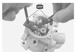
7. Make sure the valve cotters are properly seated in the groove (A).
