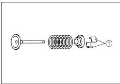
2. Remove the valve spring retainer ②, the valve spring ③. NOTE:
