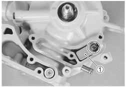
2. Install the gasket and breather plate ② to the cylinder block and secure with the three screws.
