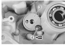
6. Install the oil pump shaft ⑤.
