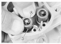
7. Make sure the retainers are properly seated in groove <sup>®</sup>.
