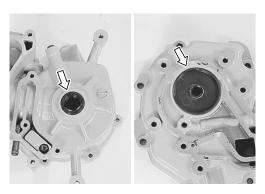
Drive the oil seal down into the position as shown in the figure.
