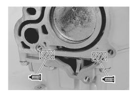
2. Insert the dowel pins ① and place a new cylinder head gasket 2 into position on cylinder.
