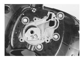
10. Remove a bolt 7 and oil seal protector 8.
