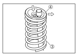
6. Push down the retainer with both thumbs to admit the valve stem into the side hole (A) of the retainer, and let it slide sidewise into the center hole.
