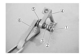
3. Install the cam rocker arm 4, the washer 5 and the cam rocker arm 6.
