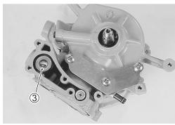
4. Apply sealant to both surfaces of thermostat cover gasket (as shown with hatched lines).
