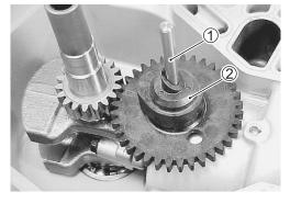
4. While aligning each mark on the camshaft gear and the crankshaft gear, install the camshaft ②.
