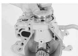
10. Remove the crankshaft fi from the cylinder block.
