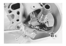
2. Install the conrod cap in the direction as shown in the figure.
