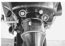
9. Remove the four bolts, then detach the power unit from the lower cover.
