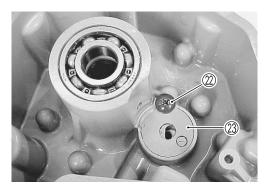
13. Remove the inner rotor ② and the outer rotor ③.
