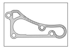
5. Install the gasket and the thermostat cover ④ to the cylinder block and secure with the four bolts.
