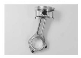
Remove piston pin circlips as shown.
