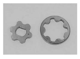
• Check oil pump case for excessive wear or damage. Replace as necessary.
