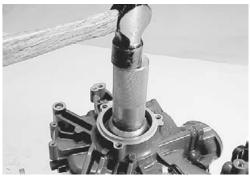
Apply engine oil to outer circumference of bearing.
