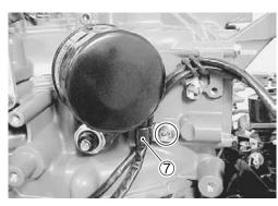
Remove the twelve (12) bolts and two (2) nuts. Remove the two (2) bolts securing front panel to crankcase. Lift up and remove power unit from oil pan.
