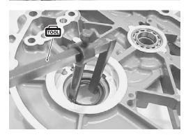
3. Apply engine oil to outer circumference of oil seal. Drive oil seal down into position as shown figure.
