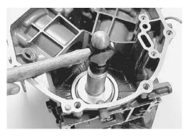
4. Apply engine oil to outer circumference of oil seal. Drive oil seal down into position as shown in figure. Do not contact oil seal to bearing.
