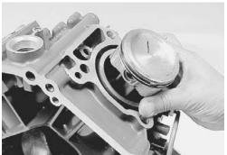
Remove two compression rings (top and 2nd) and oil ring from piston.
