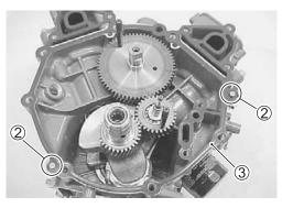
5. Place the bottom crankcase into position 4. Fit the 8 mm and 10 mm bolts of the special tool set at the positions indicated in the figure.
