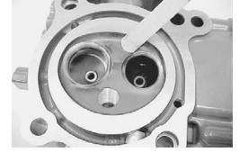
Check cylinder head for cracks in intake and exhaust ports, combustion chambers, and head surface.
