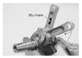
(4) Apply engine oil to conrod bolts and tighten bolt in two steps.
