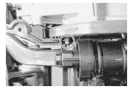
Loosen the clamp and remove the oil strainer  $\center{8}$ .
